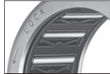
The mounted clutch engages when the housing is rotated relative to the shaft in the direction of the arrow marking [← LOCK] stamped on the cup.
