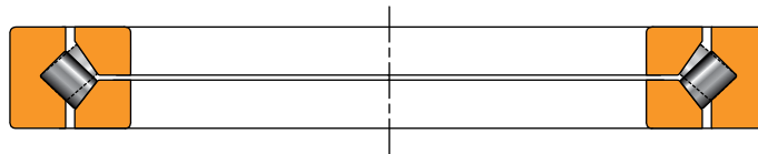
Fig. 24. Type TXR crossed roller bearings.
