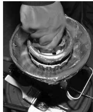
Fig. 52. Mechanical grease packer.
